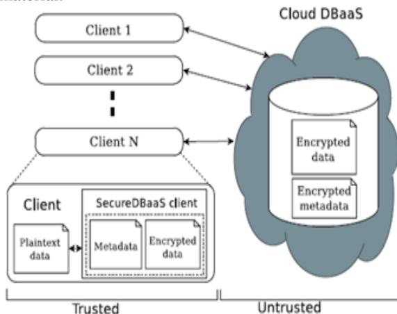
Fig.1. SecureDBaaS Architecture.
