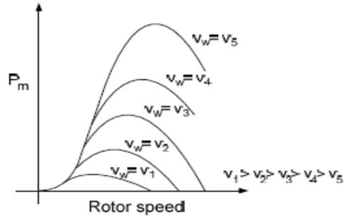
Figure6: Power Curves for a typical wind turbine
