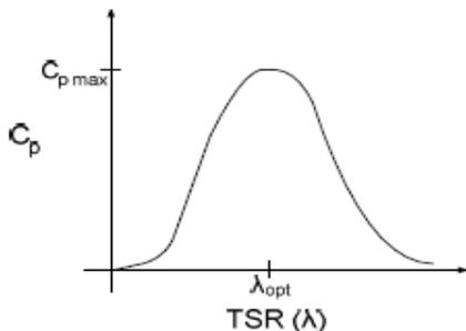
Figure5. Power Coefficient Curve for a typical turbine
